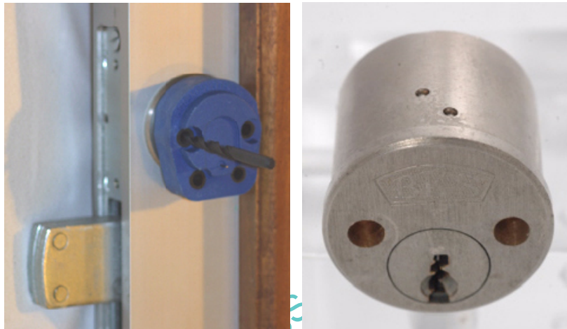
These photographs show a Peterson Mfg. drill jig for destroying set screws.
